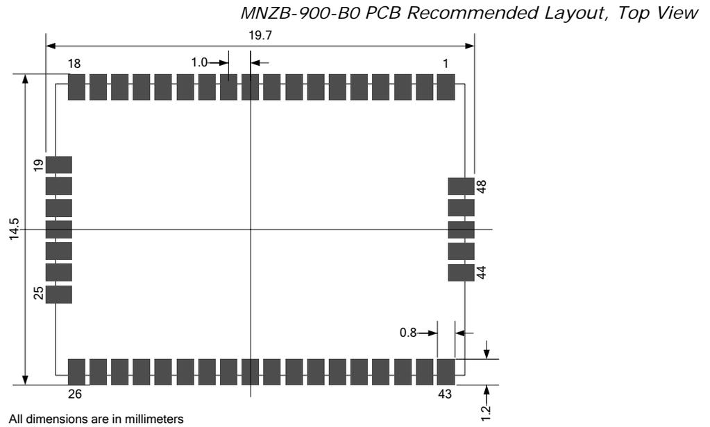
The above diagrams show the PCB layout recommended for ZigBit 900 module. Neither via-holes nor wires are allowed on the PCB upper layer in area occupied by the module. As a critical requirement, RF\_GND pins should be grounded via several holes to be located right next to pins thus minimizing inductance and preventing both mismatch and losses.
