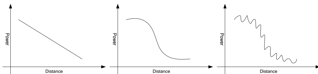
Figure 6: Theoretically vs. measured RSSI, distance given in logarithmic scale
