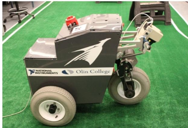
Tricycle drive is the common case in the mobile robots. It consists of one steering front wheel and two rear wheels (free wheels). The robot motion is controlled by the steering wheel's velocity  $V_F$  and the direction  $\alpha$ .
