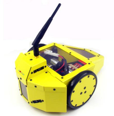
Differential drive is the common drive mechanism used in mobile robots. It consists of 2 drive wheels mounted on a common axis, and each wheel can independently being driven either forward or back-ward.
