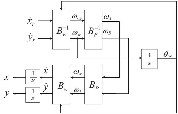
Fig. 8. Block diagram of the single wheel
