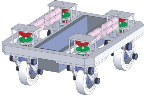
Fig. 6. Platform of the proposed omnidirectional mobile robot
