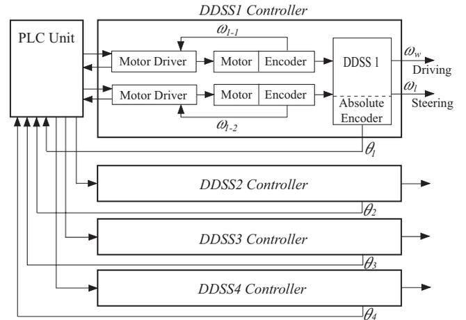
Fig. 11. Control system of the vehicle
