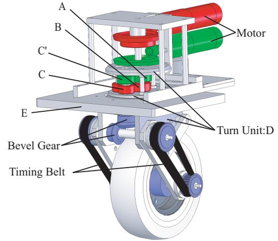
Fig. 4. Mechanism of the proposed DDSS
