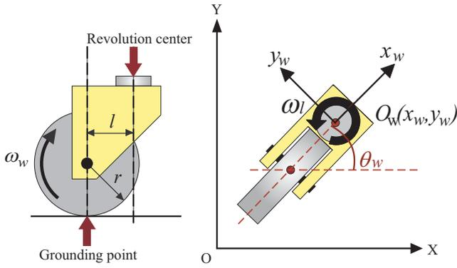
Fig. 1. Model of the caster-drive wheel
