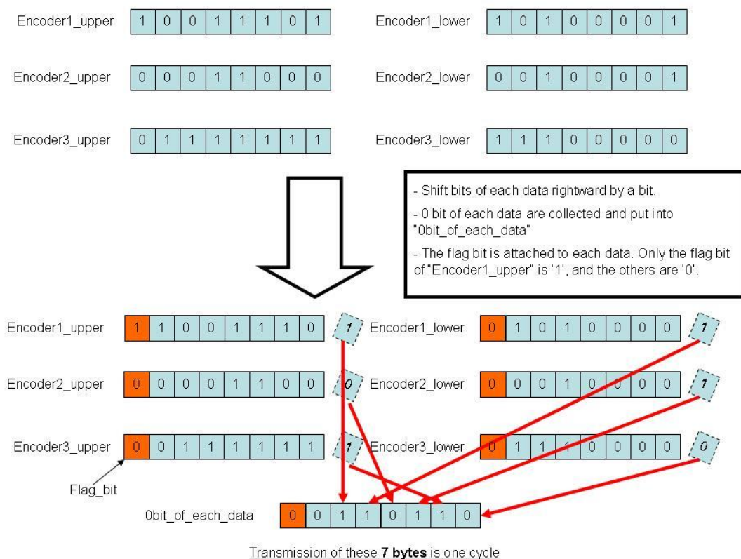
Figure 6.17 Flag attachment at PIC16F690
