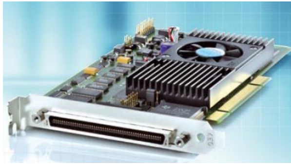
Figure 3.3 dSPACE® DS1104 R&D Controller Board [6]
