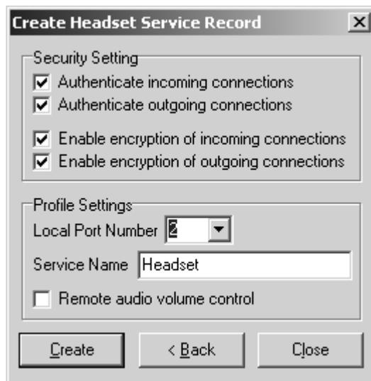
**Figure 4-12. Configuring the profile settings for headset**
