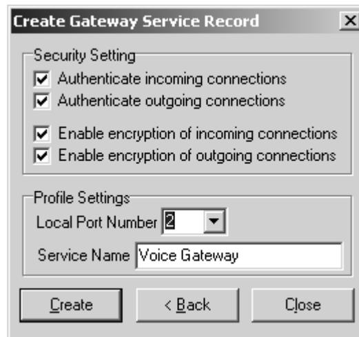
**Figure 4-26. Configuring the profile settings for HSAG**
