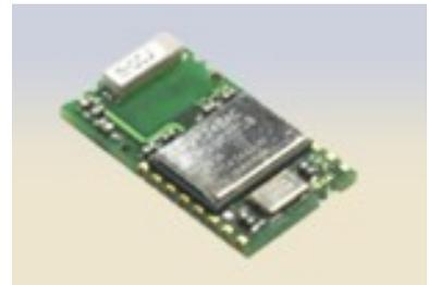
AMBER wireless provides with the BlueNiceCom 3 a Bluetooth-module with an integrated chip-antenna, based on LMX9820A from National Semiconductor. This compact and inexpensive Bluetooth-version is qualified for a serial data transmission.
