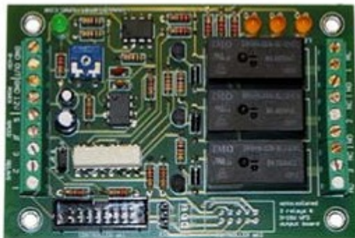
Output Board Adds Relays and VFD
