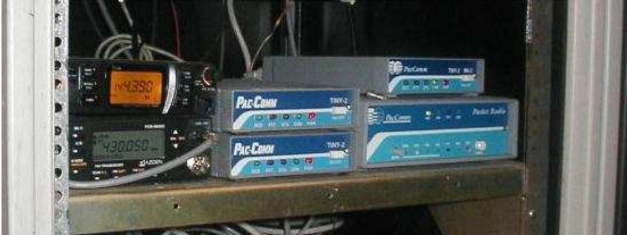
Figure 10: The WB2ZII Mic-E Digipeater at the Jail (and one of the UHF packet digis)
