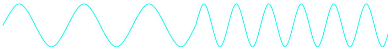
Figure 1: AFSK waveform
