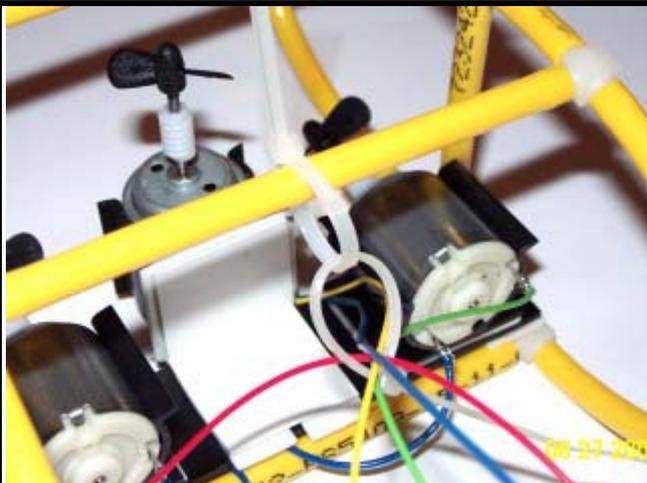
6. Take one short white cable tie and loop it loosely over the top stern strut. Attach the wire bundle using another white cable tie to the first tie, like the links of a chain.
