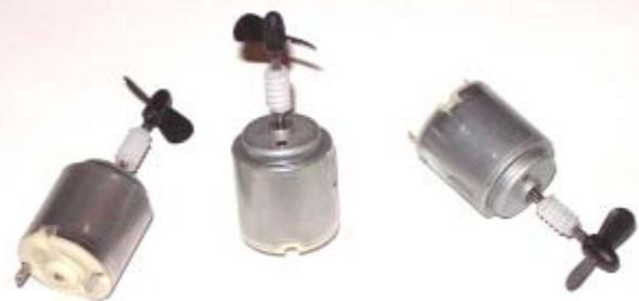
2. Push the propeller assemblies firmly onto the shafts of the motors.
