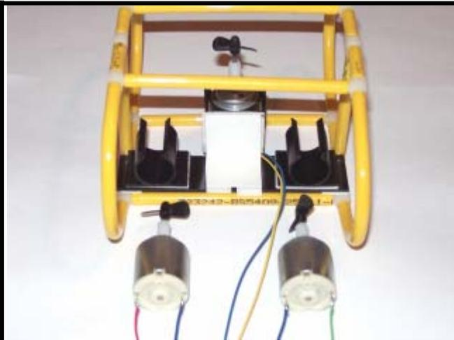
4. Clip the vertical thruster (with the yellow wire) into the middle position, bringing the wires backward to the stern of the ROV.
