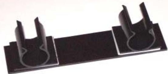
**6.** Peel the backing off the sticky tabs and fix the clips to the plate as shown. They should be about 3mm to 5mm in from the ends.
