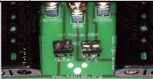
3. Solder the terminal blocks to the board such that the screw holes are oriented towards the closest edge of the board (towards the 3 larger holes in the board).
