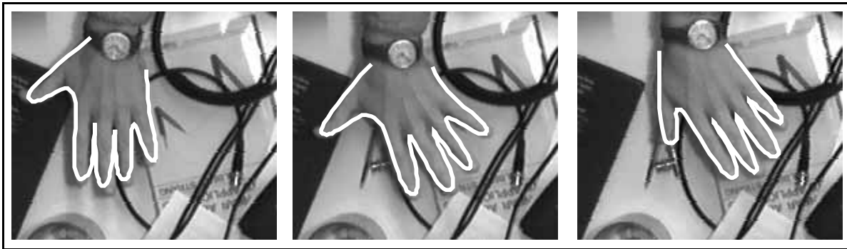
Figure 16: Tracking a flexing hand across a cluttered desk. Representative stills from a 500 field (10 second) sequence show a hand moving over a highly cluttered desk scene. The fingers and thumb flex independently, and the hand translates and rotates. Here the CONDENSATION algorithm uses N = 1500 samples per time-step initially, dropping gradually over 4 fields to N = 500 for the tracking of the remainder of the sequence. The mean configuration of the contour is displayed.
