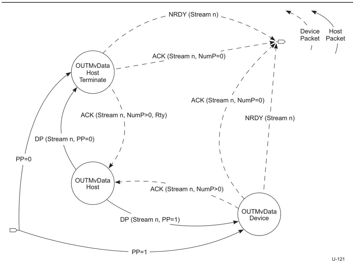
**Figure 8-32. OUT Move Data State Machine (OMDSM)**
