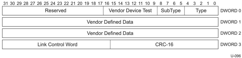
Figure 8-7. Vendor Device Test LMP
