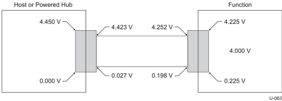
Figure 11-5. Worst-case Voltage Drop Topology (Steady State)
