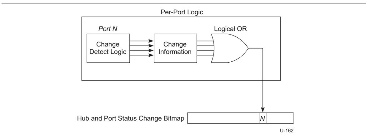
**Figure 10-24. Example Hub and Port Change Bit Sampling**
