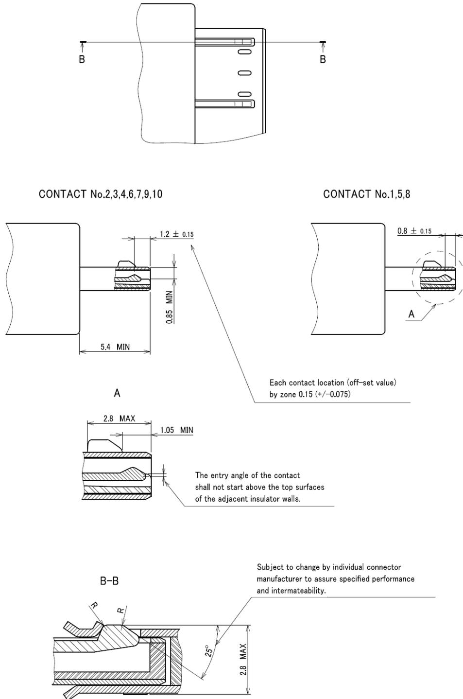
Figure 5-13. USB 3.0 Micro-B and Micro-A Plug Interface Dimensions
