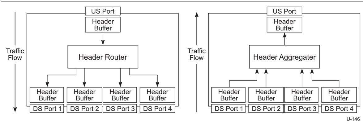
Figure 10-7. Typical Hub Header Packet Buffer Architecture
