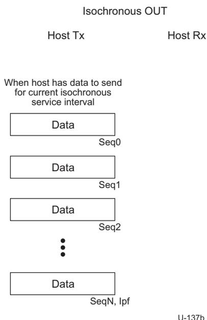
**Figure 8-47. Isochronous OUT Transaction Format**
