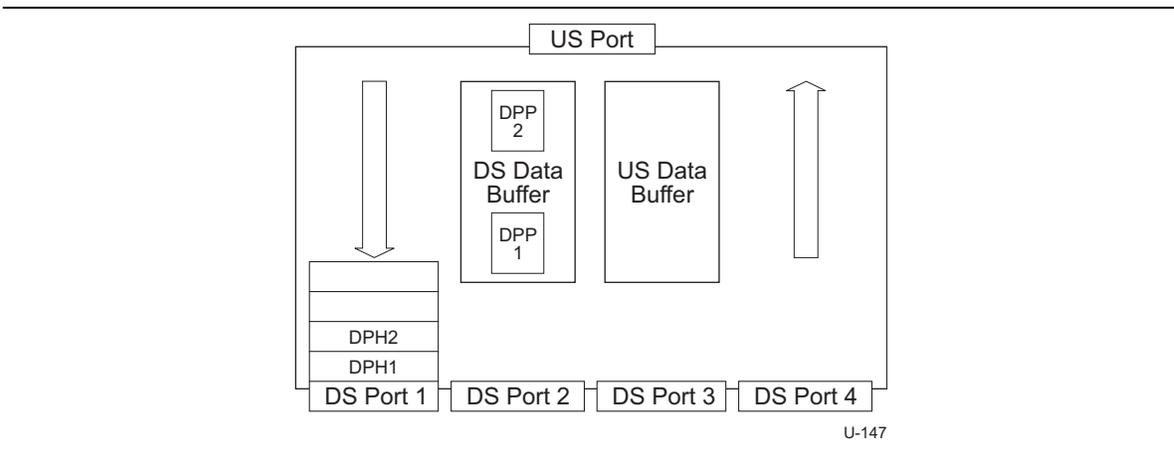
Figure 10-8. Hub Data Buffer Traffic (Header Packet Buffer Only Shown for DS Port 1)
