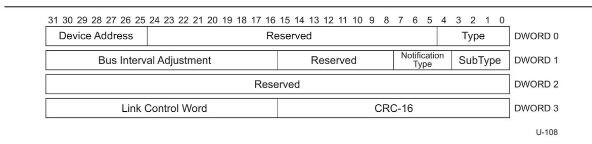
**Figure 8-19. Bus Interval Adjustment Message Device Notification**
