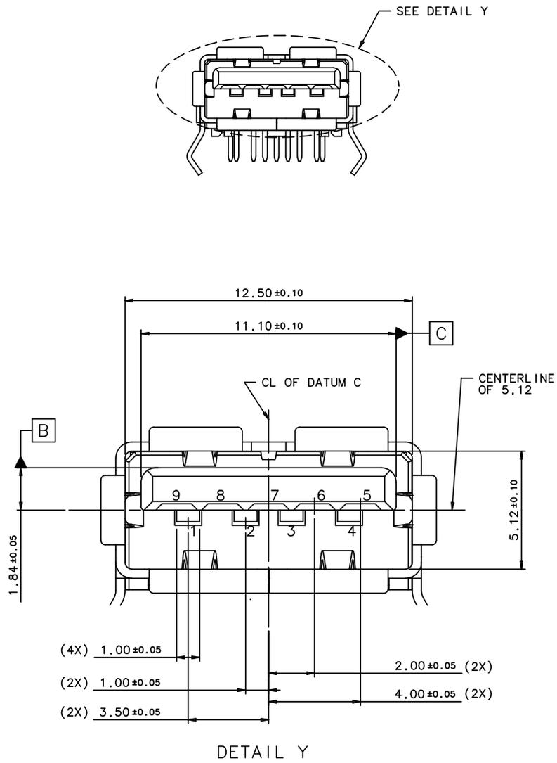
Figure 5-1. USB 3.0 Standard-A Receptacle Interface Dimensions
