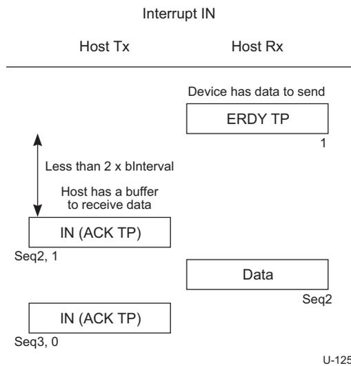
**Figure 8-37. Host Resumes IN Transaction after Device Sent ERDY**
