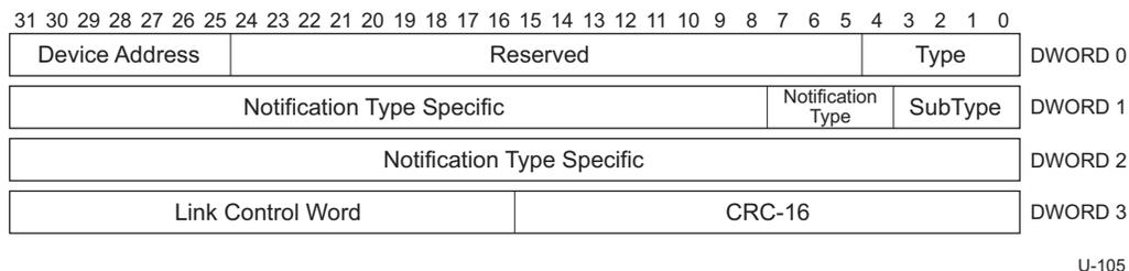
Figure 8-16. Device Notification Transaction Packet
