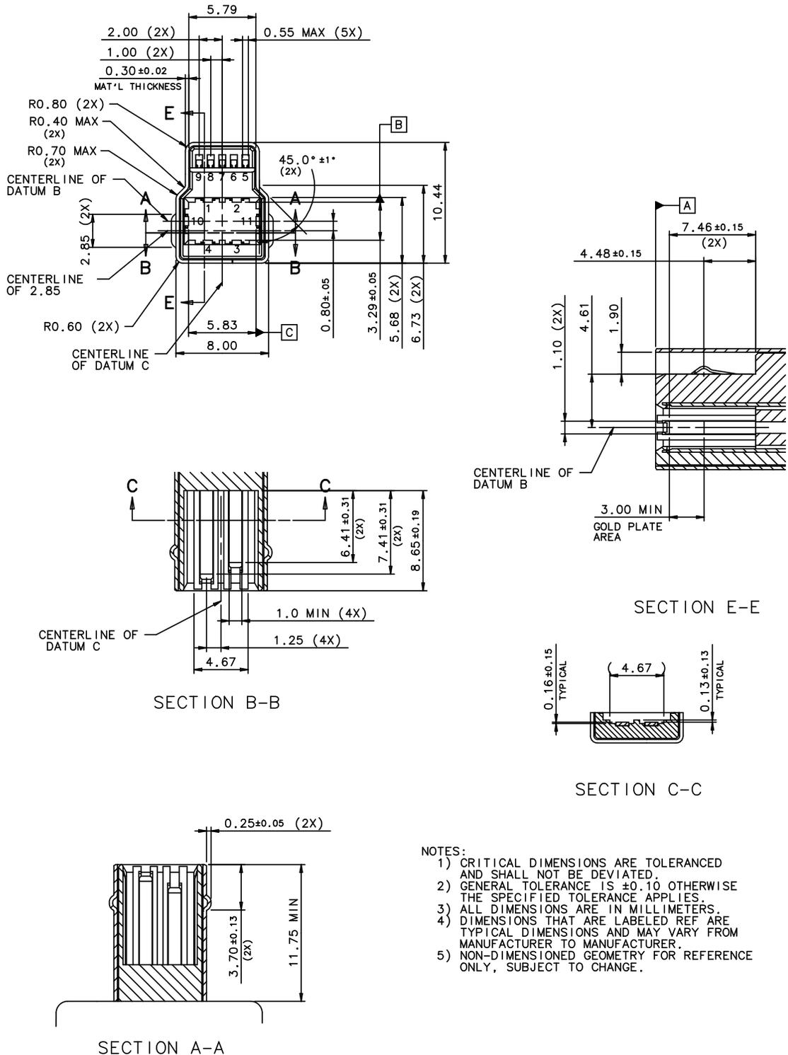
Figure 5-10. USB 3.0 Powered-B Plug Interface Dimensions
