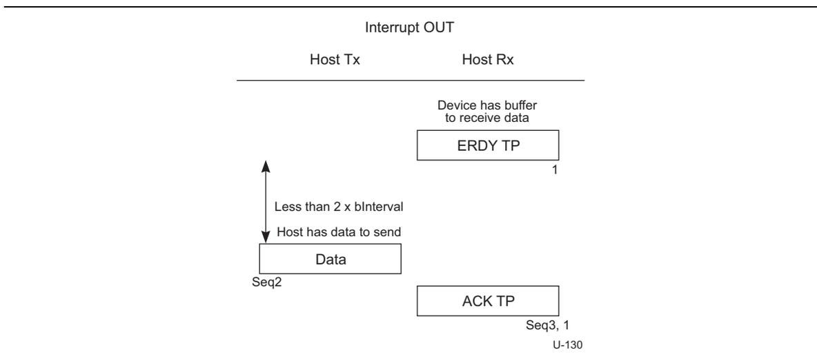
**Figure 8-42. Host Resumes Sending Interrupt OUT Transaction After Device Sent ERDY**
