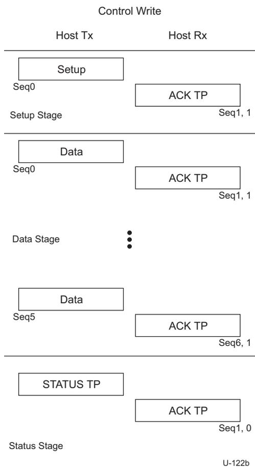
**Figure 8-34. Control Write Sequence**
