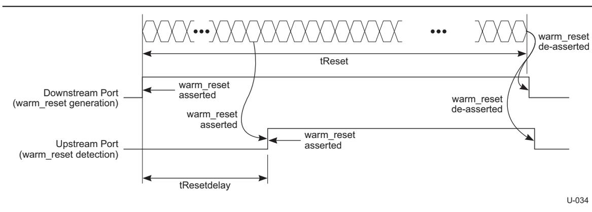
Figure 6-22. Example of Warm Reset Out of U3
