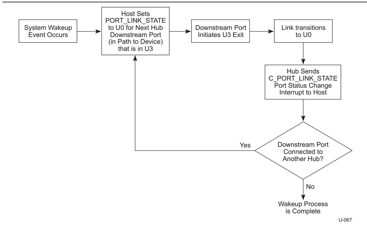
Figure C-1. Flow Diagram for Host Initiated Wakeup
