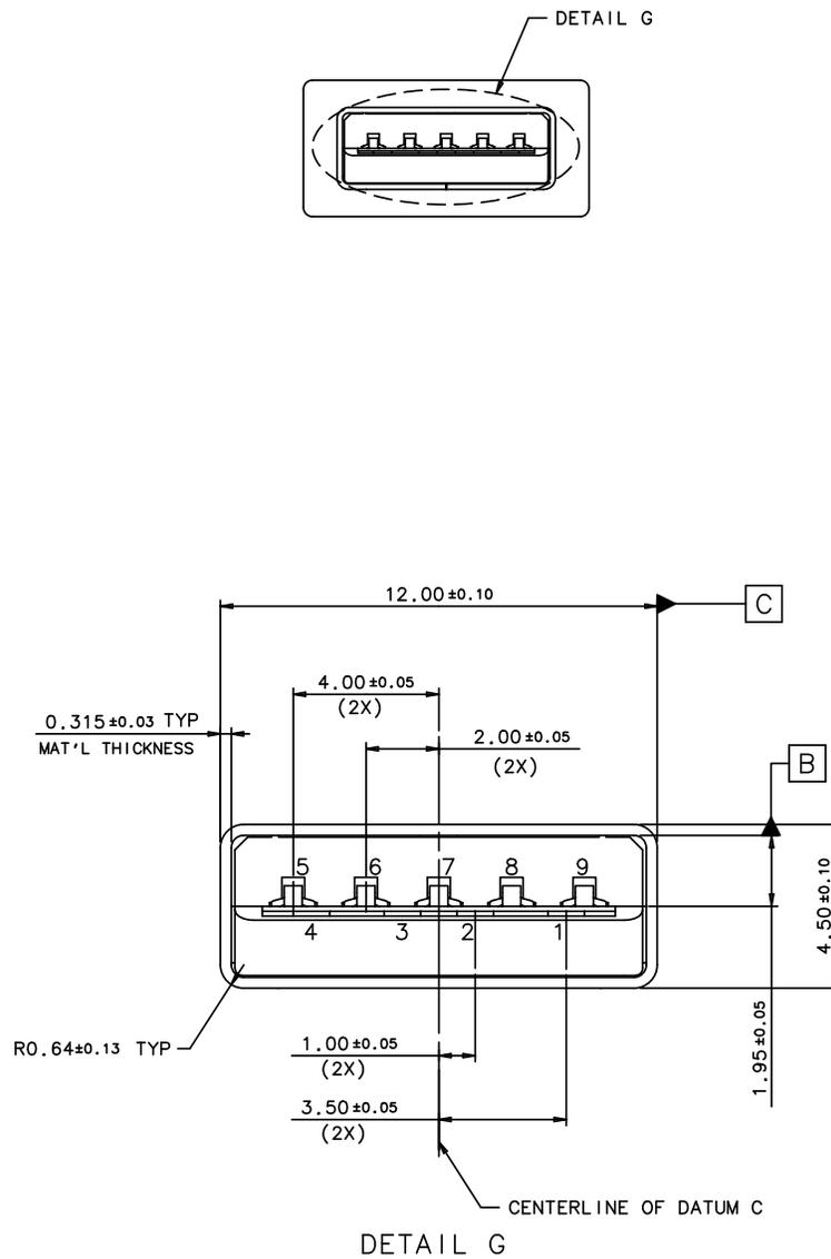
Figure 5-2. USB 3.0 Standard-A Plug Interface Dimensions
