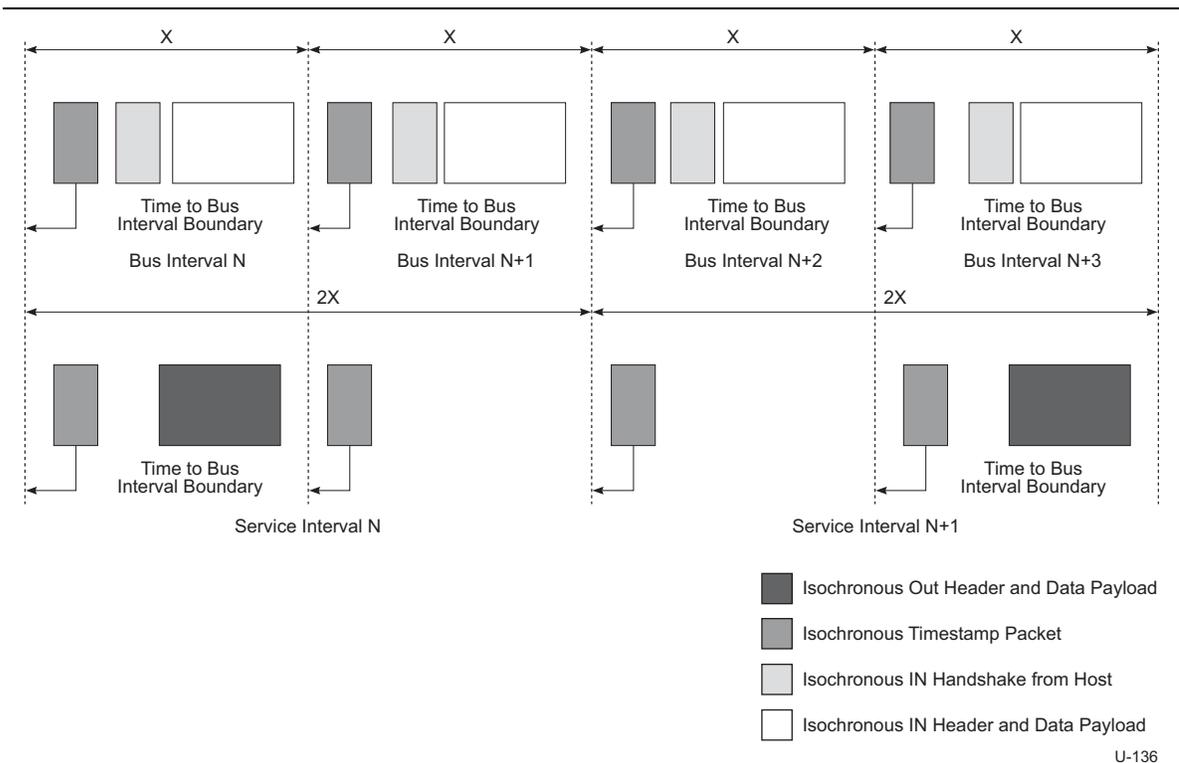
**Figure 8-45. Multiple Active Isochronous Endpoints with Aligned Service Interval Boundaries**
