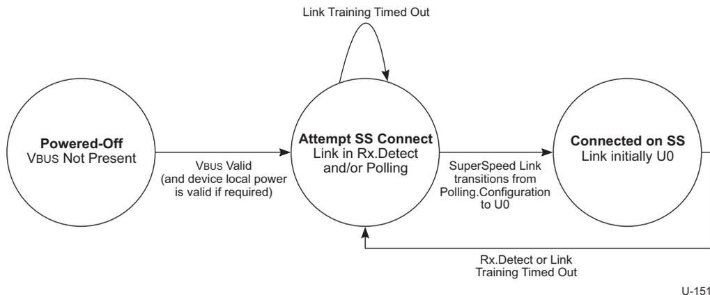
Figure 10-12. Hub Connect State Machine
