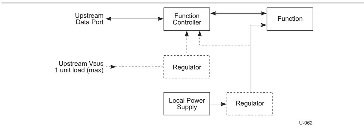
Figure 11-4. Self-powered Function
