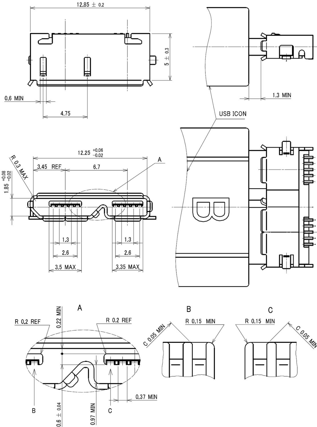
NOTE : General tolerance is  $\pm 0.05$  mm, otherwise the specified tolerances apply.
