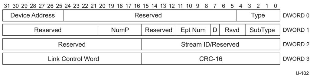
Figure 8-13. ERDY Transaction Packet
