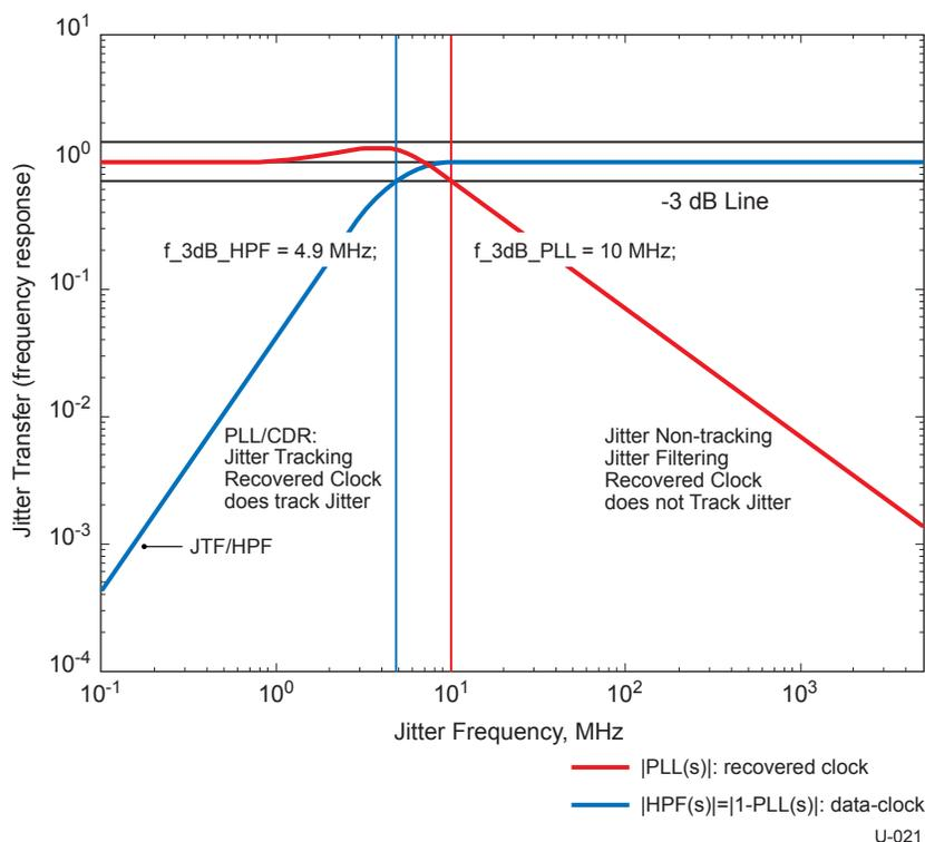
Figure 6-9. “Golden PLL” and Jitter Transfer Functions
