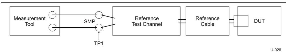
**Figure 6-14. Tx Normative Setup with Reference Channel**
