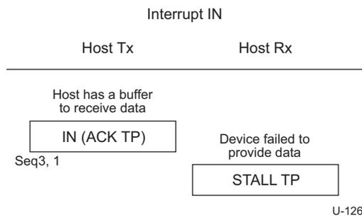
**Figure 8-38. Endpoint Sends STALL TP**
