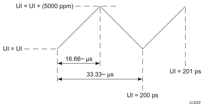
**Figure 6-10. Period Modulation from Triangular SSC**
