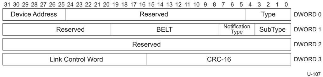
Figure 8-18. Latency Tolerance Message Device Notification
