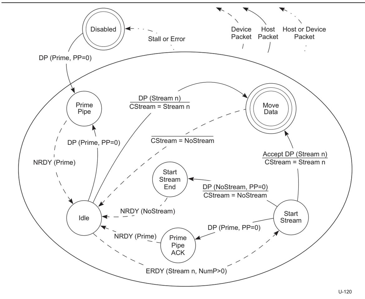
Figure 8-31. OUT Stream Protocol State Machine (OSPSM)
