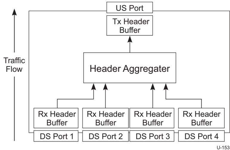
**Figure 10-15. Example Hub Header Packet Buffer Architecture - Upstream Traffic**
