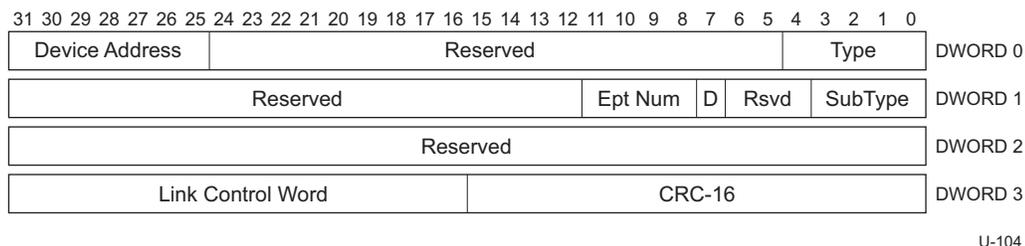
Figure 8-15. STALL Transaction Packet
