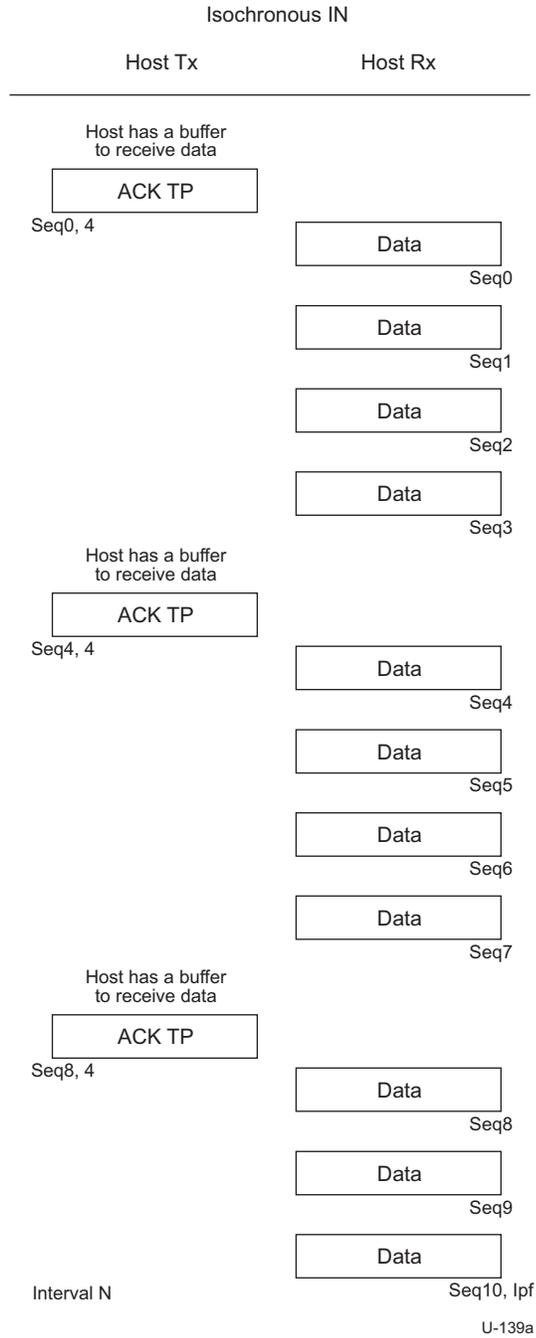
**Figure 8-50. Isochronous IN Transaction Example**
