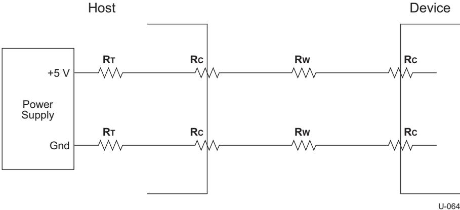
Figure 11-6. Worst-case Voltage Drop Analysis Using Equivalent Resistance
