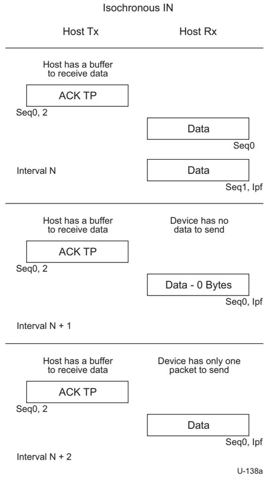
**Figure 8-48. Sample Isochronous IN Transaction**
