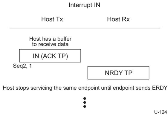
**Figure 8-36. Host Stops Servicing Interrupt IN Transaction Once NRDY is Received**
